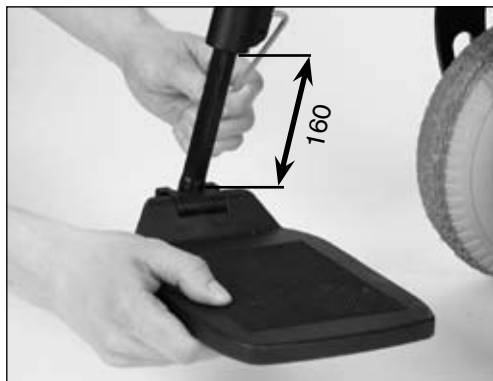
Fig. 11 Adjusting the lower leg length
