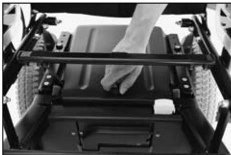
Fig. 16 Remove battery cover
