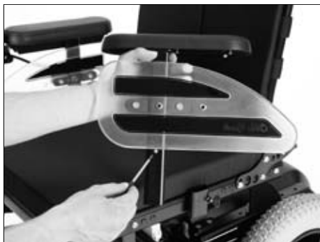
Fig. 8 Adjusting the height of the armrest
