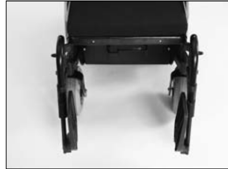
Fig. 12 Footplates flipped up
